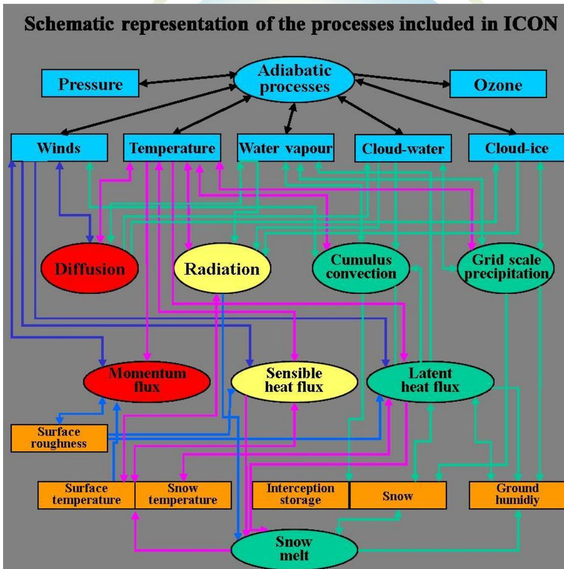
Figure 2: A schematic of the main processes included in ICON model. (Courtesy: DWD)
