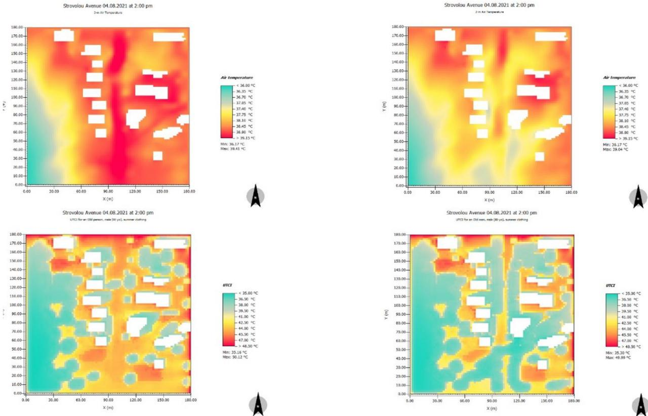
Figure 15: ENVI-met implementation for Nicosia. Simulated air temperature (top) and UTCI comfort index (bottom) for control/current (left) and heat mitigation greener space scenario (right). White rectangles indicate built-up areas.
