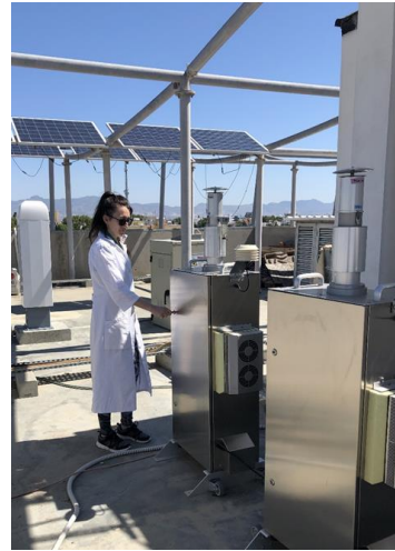
Figure.2.3.1 Left : spore trap for pollen and fungal spores sampling. Right : total suspended particulates with sequential sampler for bacteria
