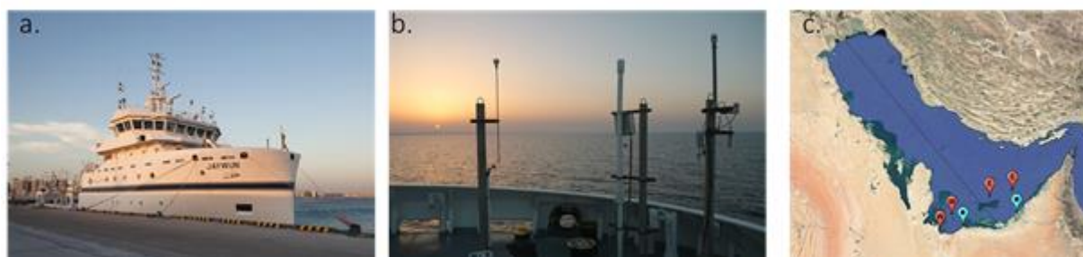
Figure 4.2.2.1 : a. The research ship vessel of Environment Agency Abu Dhabi used, b. the inlets of NMHC, reactive and greenhouse gases, and c. the anchoring locations (in red) and the ports (in cyan) sampled throughout the campaign.
