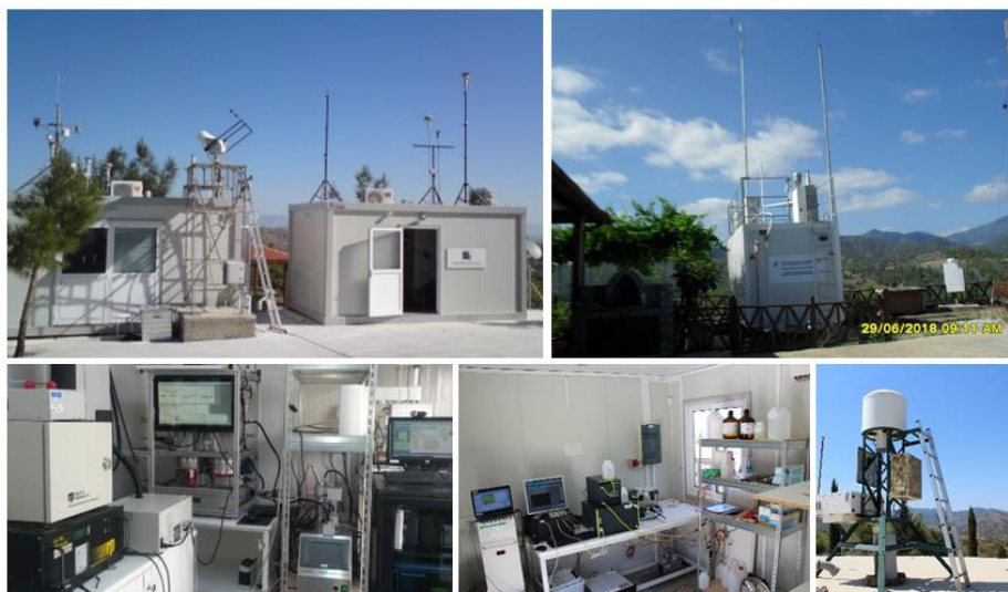
Figure 8 - The AMX station consisting of two containers for aerosol measurements and an EMEP container for trace gas and meteorological measurements.
